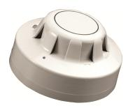
The Series 65 Optical Smoke Detector uses light sensing technology to "see" smoke entering the chamber. The external detector moulding is identical to that of the ionisation detector and has an indicator LED which is clear in quiescent state and produces a red light in alarm.
